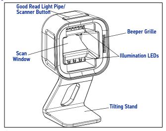
Figure 2. Scanner Features - Bottom View
